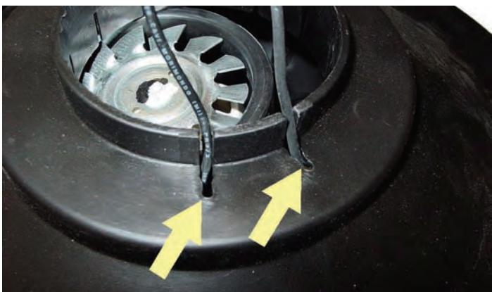
→ Pull the connecting cable of the suction turbine out of the cable slots (arrows).
