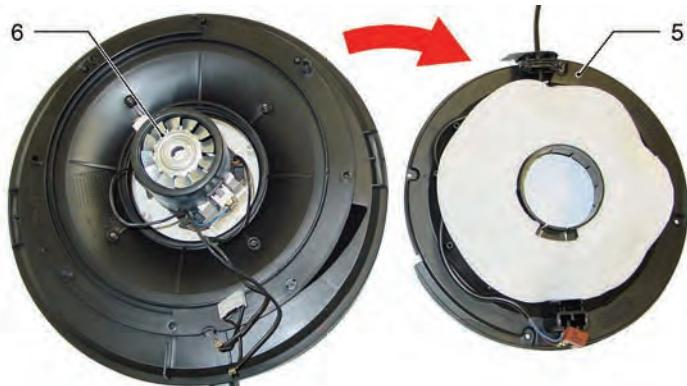
→ Remove the cover (5) from the suction turbine casing.
