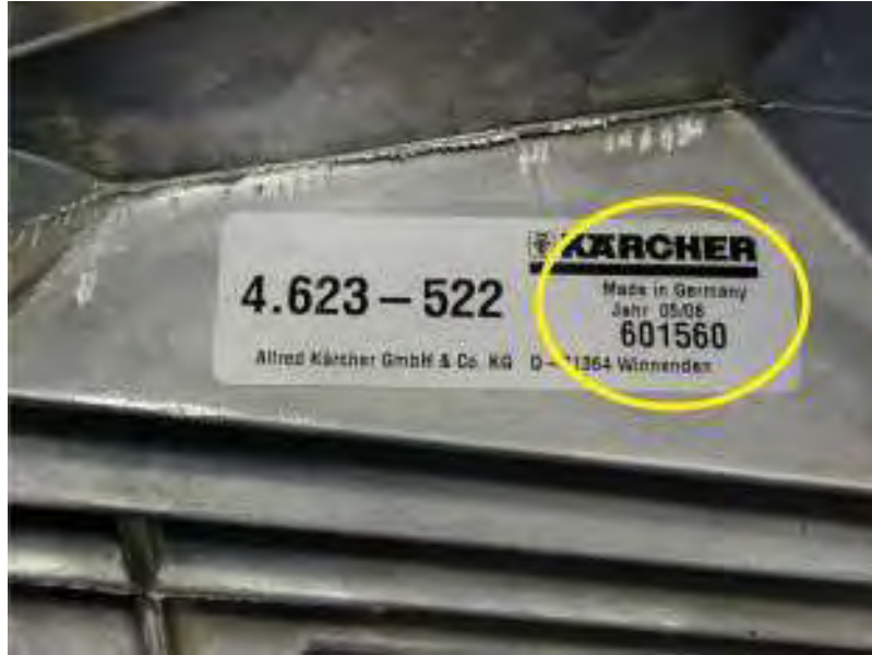
Fig. 2: Motor nameplate with production date (example 05/08)
