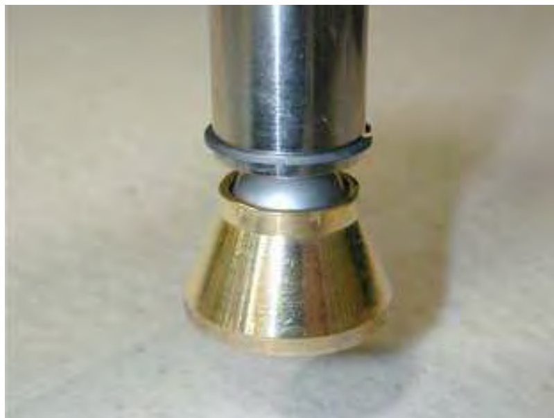
Fig. 1: Piston with piston shoe pressed on
