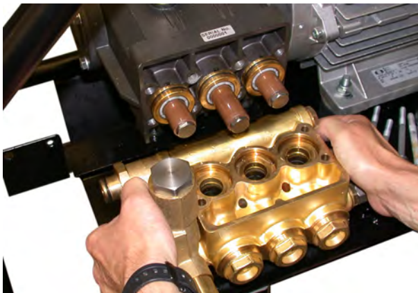
The removed cylinder head cross section seal setup, see pump diagram.
