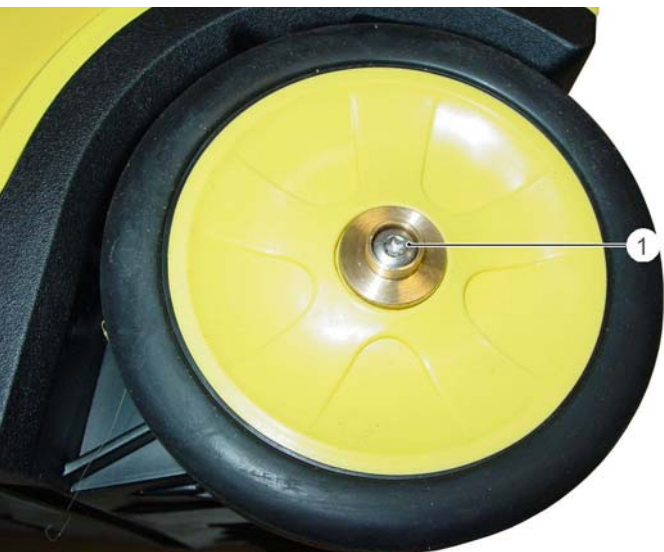
1 Fastening screws (2x), wheel mount
