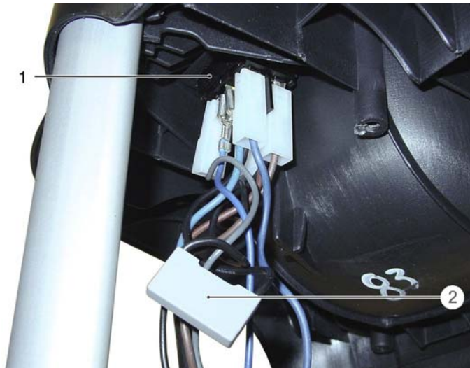
1 Main switch for brushing/vacuuming operations 2 De-interference capacitor
