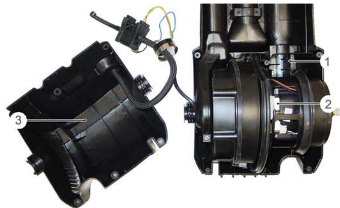
1 Bottom half bearing, suction turbine housing 2 Suction turbine (M1) 3 Top half bearing, suction turbine housing
