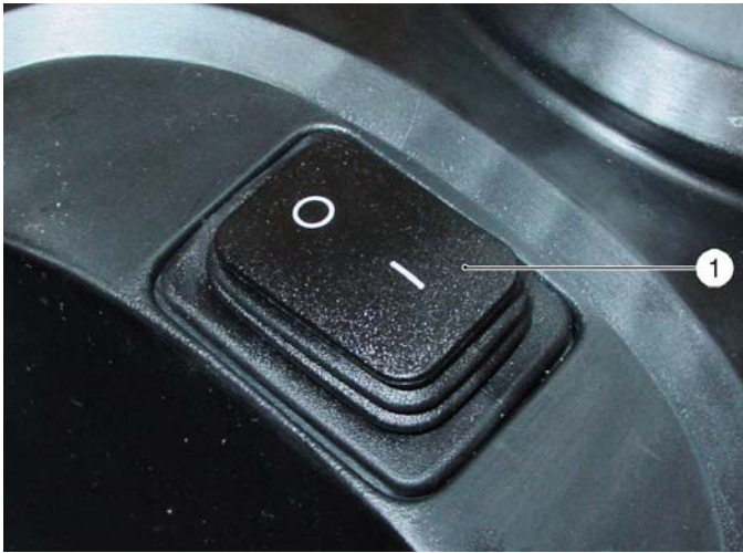
1 Main switch for brushing/vacuuming operations
