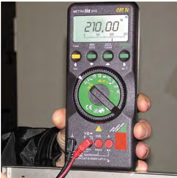
Frequency measurement with multimeter
