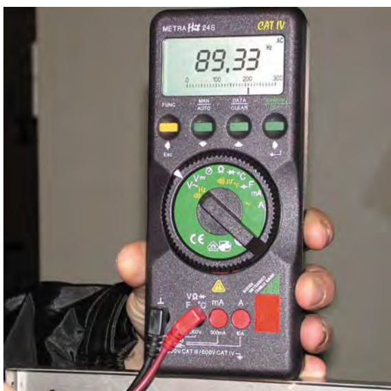
Frequency measurement with multimeter
