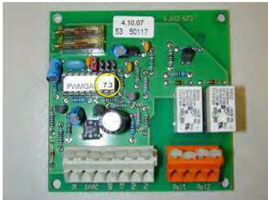
Fig. 1: PWM electronics module (6.682-673) in the latest version with software version 7.3 (encircled)
