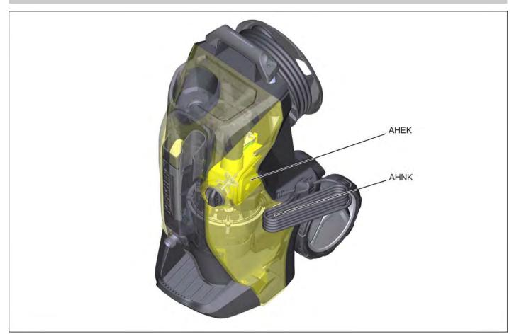
AHEK Uninstall / install electrical box AHNK Uninstalling / installing mains connection
