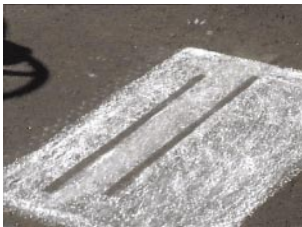
Scrubbing pattern on floor coated with chalk
