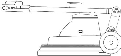
With the 230V/60Hz variant the handle can be swivelled to the front for transport and storage.
