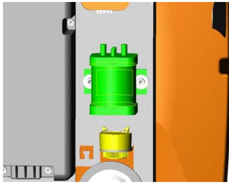
Picture 29: Power relay
