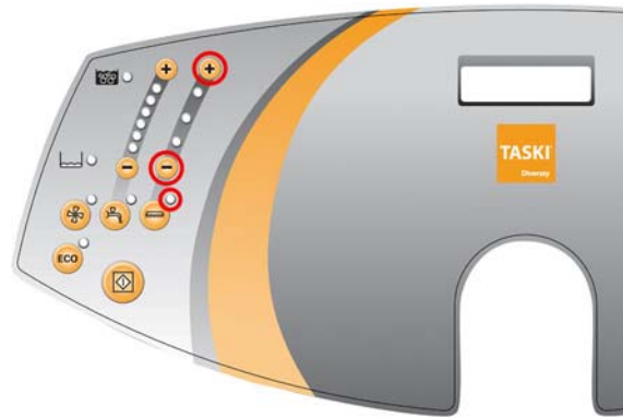
Picture 11: Brush pressure dosing (+) and (-)
