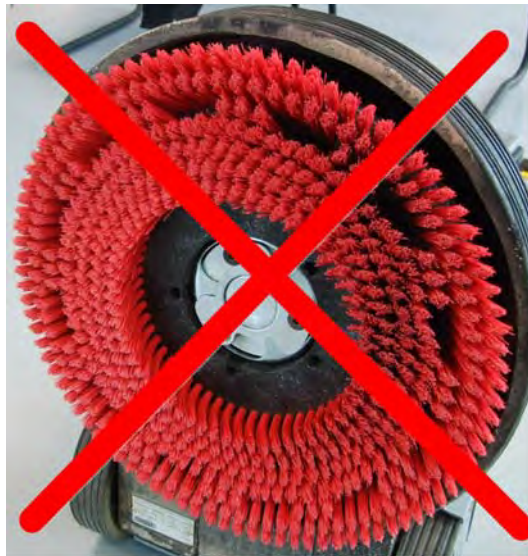
Fig.: Brushes must not be used in the high speed mode.
