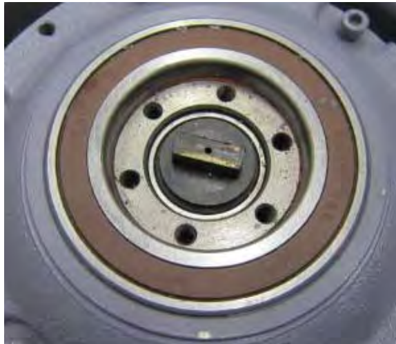
Figure: Coupling element with rubber-coated segments.
