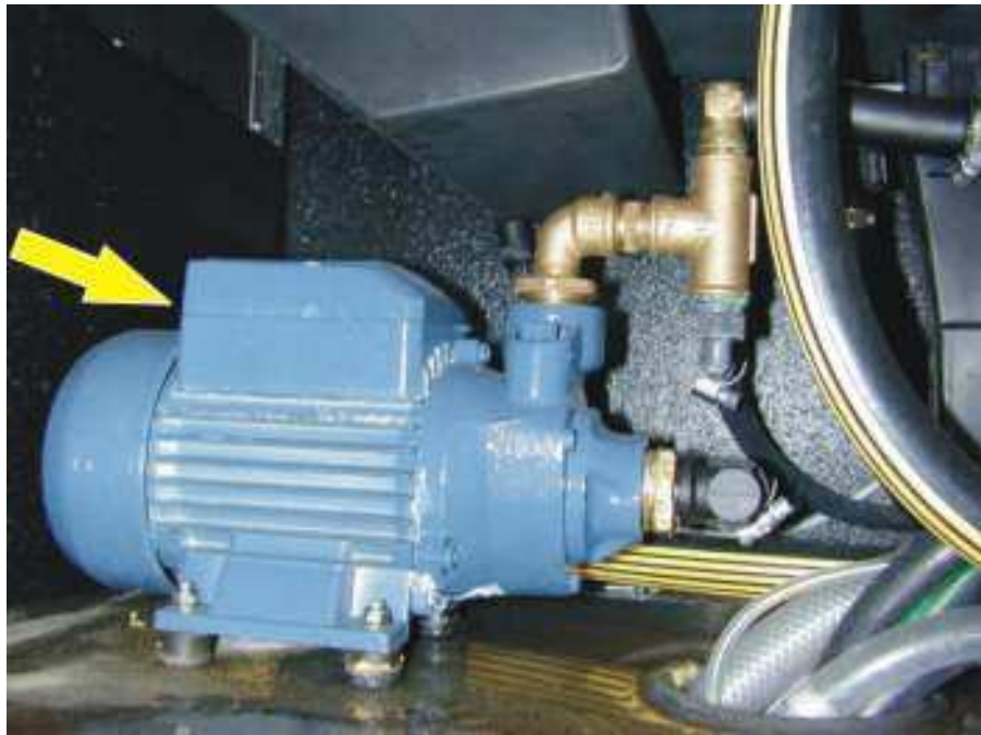
Fig. 2: Seal (6.984-606) between motor and the lid of the terminal box
