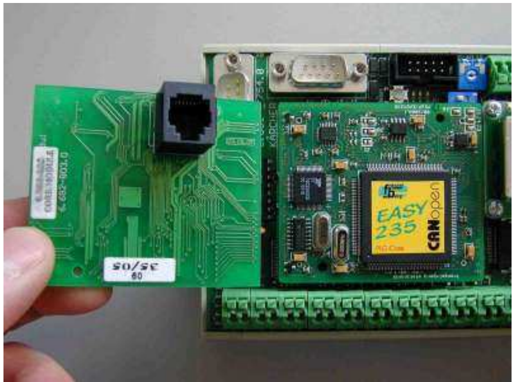
Figure 1: Printed circuit board (6.682-754) with processor module. Left: new processor module (6.682-803). When attaching, mind the correct position!
