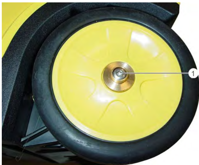
1 Fastening screws (2x), wheel mount
