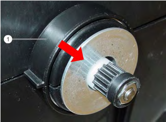
1 Bearing ring (2x), axle
