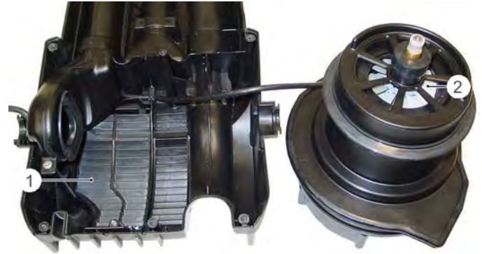
1 Bottom half bearing, suction turbine housing 2 Suction turbine (M1)
