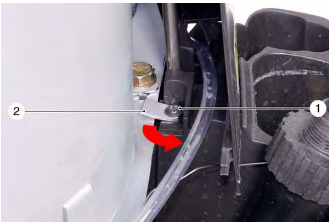
1 Screw 2 Holding plate
