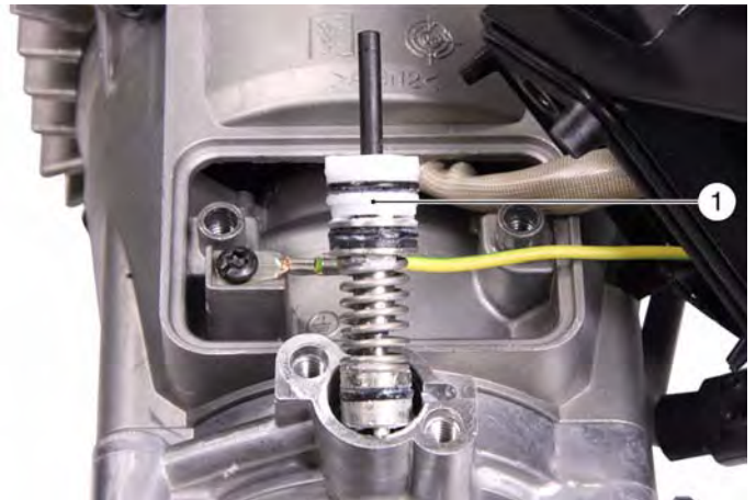
1 Overflow valve (control piston, pressure switch)
