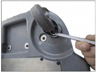
ABRH Uninstall / install wheels in the back
