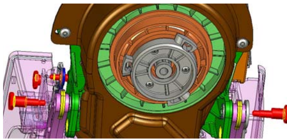
Picture 70: Brush drive mounting detail
