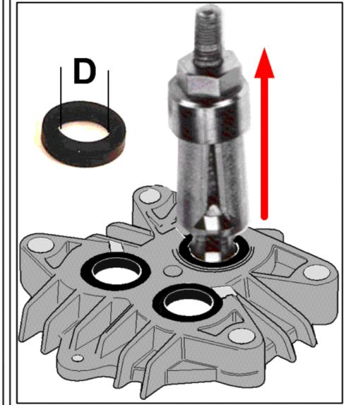
**210 Tool countersupport internal puller**
