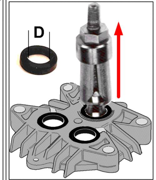
**208 Tool internal puller D5-8mm**
