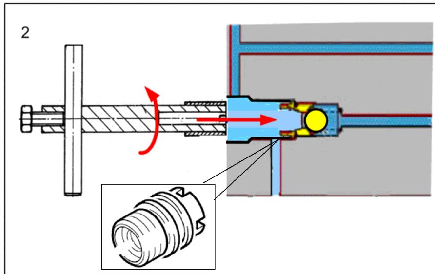
**203 Tool valve seat excess-current**
