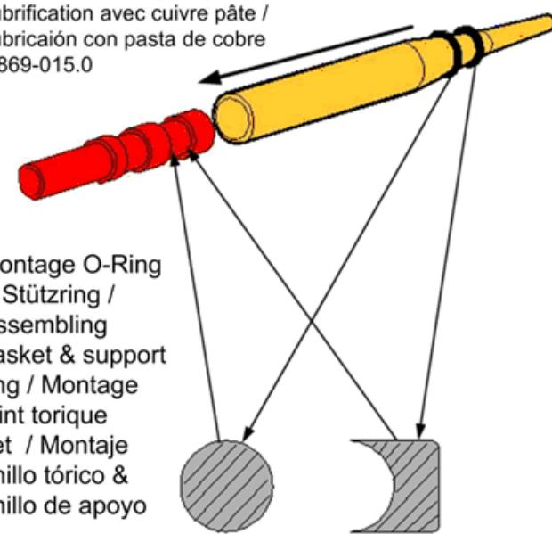
**205 Tool support mandrel O-Ring seal -D9,0mm**
