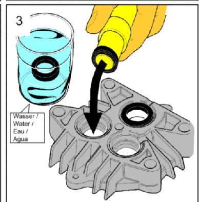
**211 Tool mandril grooved rings -Piston D14mm**
