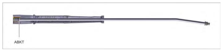
ABKT Uninstalling / installing the ball bearing spray lance
