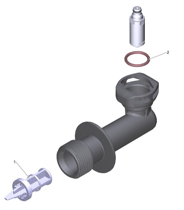
901 Suction cover for replacement with SV5 ( (4.063-913.0) Home and Garden \ High pressure cleaner cold water \ Electric motor \ K 3 \ K 3 Car & Home \*EU \ Spare parts list K3 Car& Home \*EU \ Pump set complete K3 FC/MR \*EU (0,8kW) \ Pump set RV upr. K3 \*EU (0,8kW) \ Suction cover
