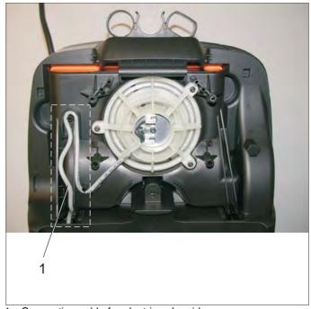
Connecting cable for electric solenoid
