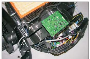
**Note:** Surface A of the hood and surface B of the turbine housing must touch each other once installed.
