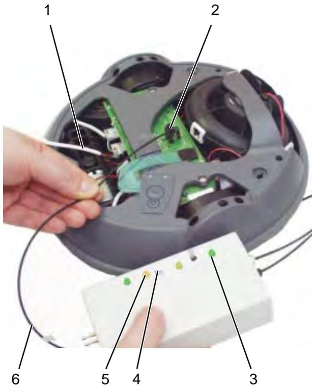
For the „Infrared sensor“ test item it is necessary to simulate the infrared beams of the charging station using the test unit.
