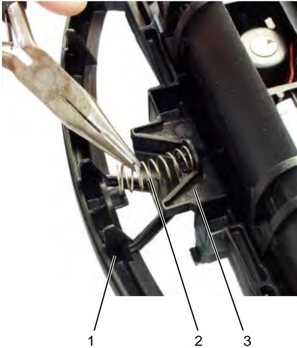
**Remove compression and tension springs**
