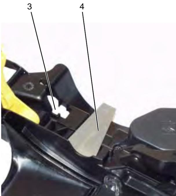
The leaf spring (4) always pushes the drive motors (1x each left and right) evenly to the ground.
