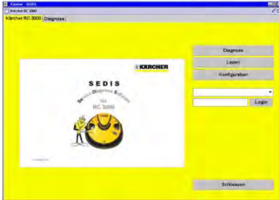
„SEDIS“, the **S**ervice **D**iagnostic **S**oftware, allows all electrical components of the robot to be checked for defects on a laptop using a service cable and offers repair solutions.
