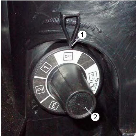
Service switch in „OFF“ position
