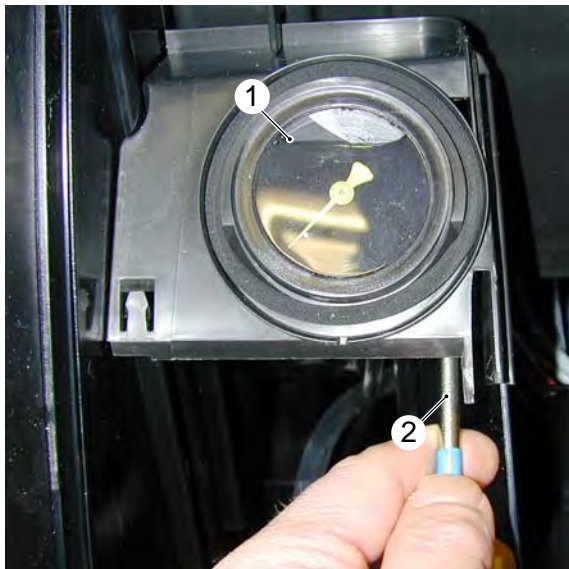
Push in right-hand retaining clip with screwdriver.
