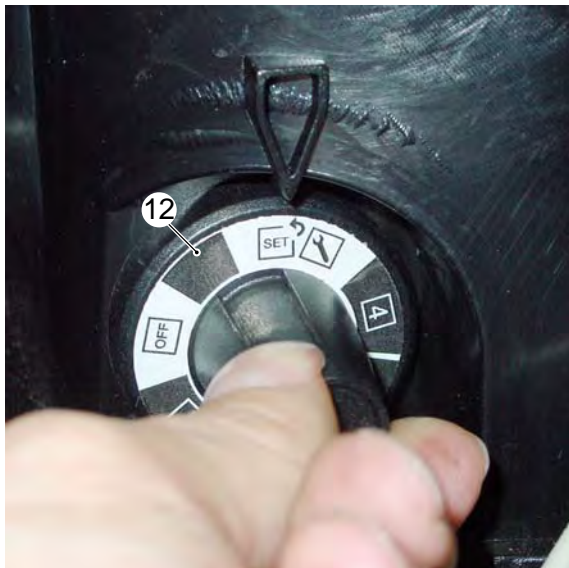
Change the setting using the Service switch
