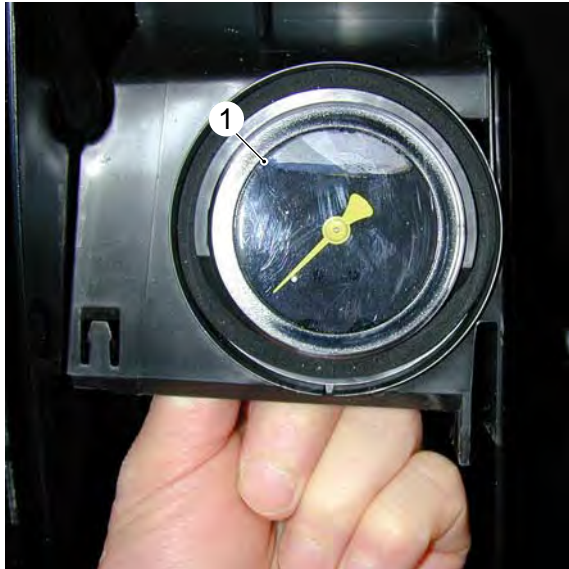
Push in left-hand retaining clip by hand.
