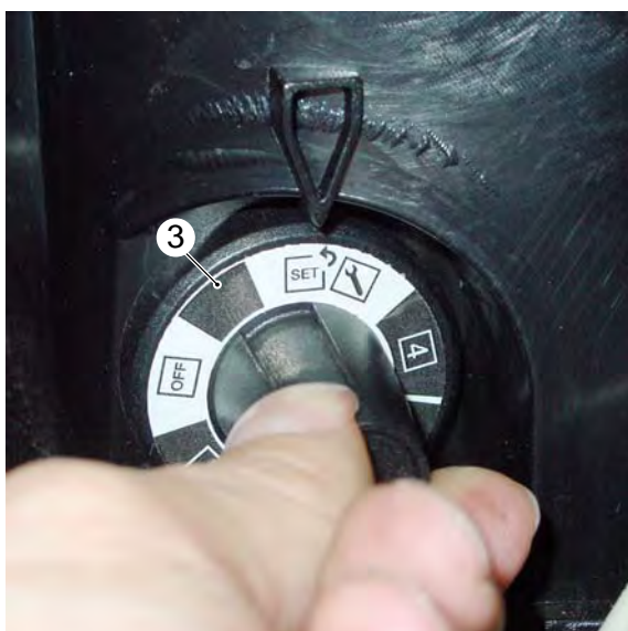
Change the setting using the Service switch
