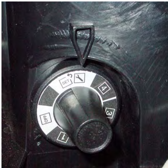
Service switch in „Service“ position
