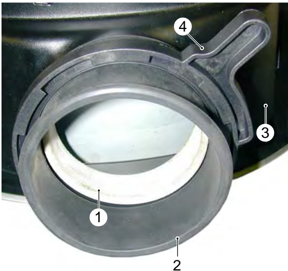
Installed clamping ring with rubber collar locking lever
