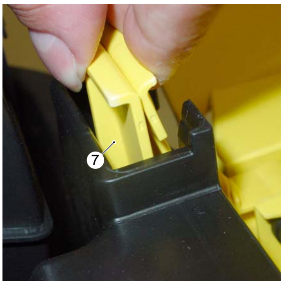
Unclip unit cover hinge
