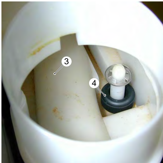
Scale inhibitor tank with level sensor
