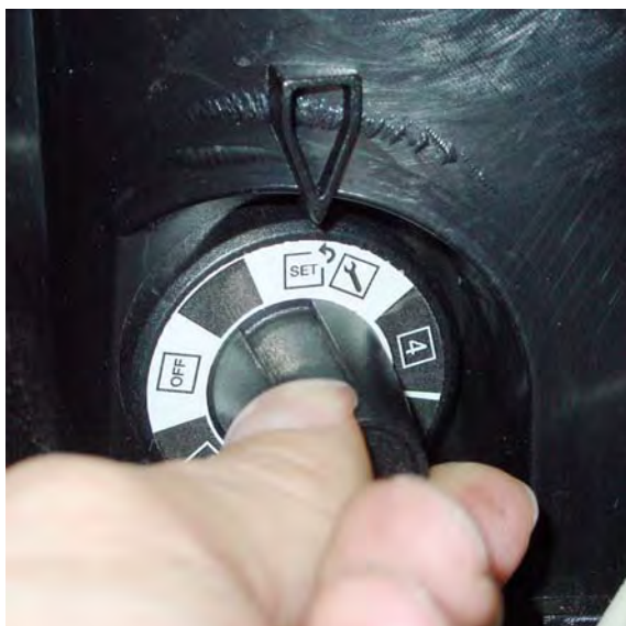
Service switch in „SET“ position
