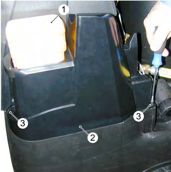
Top RFID unit with inserted scale inhibitor bottle
