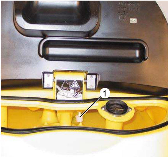
Float switch (S17), dirty water tank open
