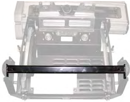
Position of the support strut - appliance hood removed for clarity.
