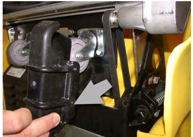
Position of the support strut - appliance hood removed for clarity.
