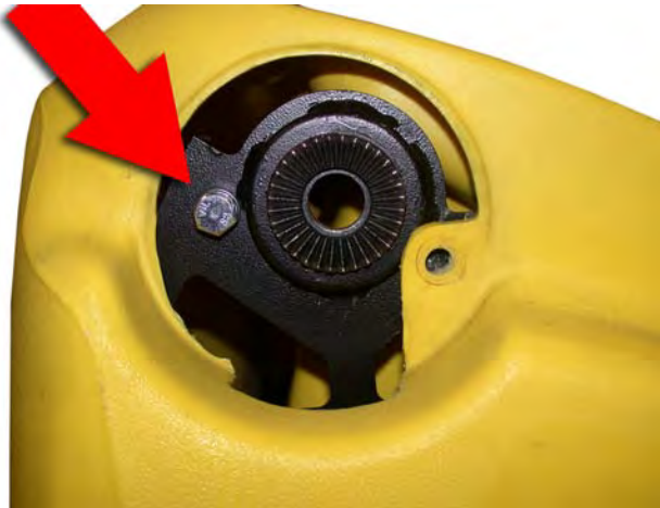
Position of the support strut - appliance hood removed for clarity.
